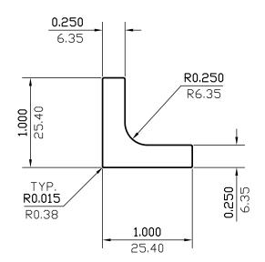
0.250(3.18)WALL THICKNESS EXCEPT AS SHOWN DATE REV DESCRIPTION BY 03/20/23 REMOVED ALLOY NDZAL мм.2 IN.<sup>2</sup> 290.757 0.451 EST.AREA EST.AREA 0.791 0.532 EST.WT. LBS/FT. EST.WT. KG/M. 3.861 98.057 EST.PER. MM. EST.PER. OUT PER. OUT PER. MM. 1.402 C.C.D. 35.605 C.C.D. MM. M/F FINISH ALLOY DWN BY C.P. SCALE 1:1 03/30/2009 CKD BY FACTOR DATE
